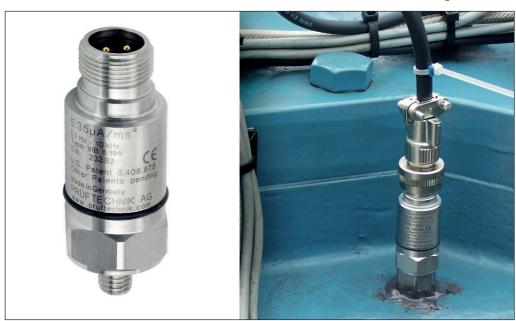
Accelerometers of the VIB 6.195 series are used for the measurement of absolute casing vibrations on machinery with rotating components. Due to the very low limit frequency, the accelerometers are particularly suitable for very slowly rotating components ( $n \ge 6$  rpm) such as the main bearings of a wind turbine.
