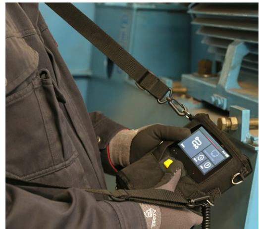
Shoulder strap and hand straps can be adjusted for left- or right-handed operation.
