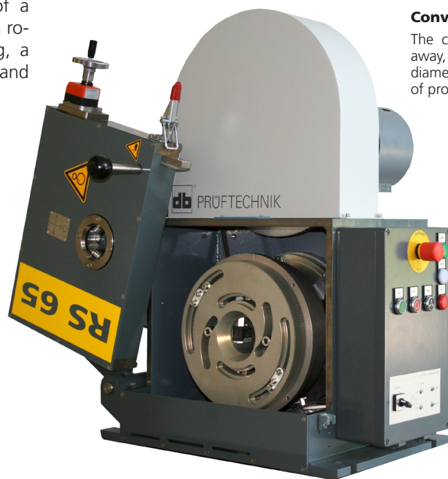
Photo from right to left: Combined offline testing with RS65 rotation system and encircling coil in magnetization unit followed by DC and AC demagnetization units.
