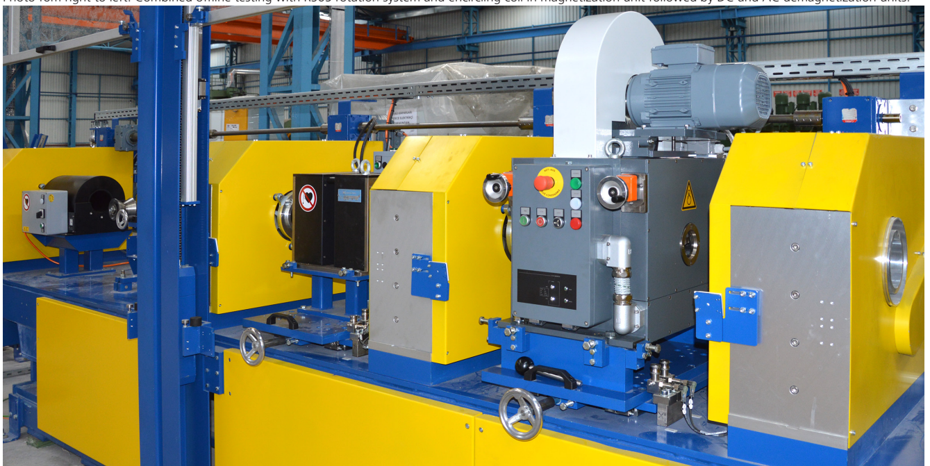
Photo from right to left: Combined offline testing with RS65 rotation system and encircling coil in magnetization unit followed by DC and AC demagnetization units.
