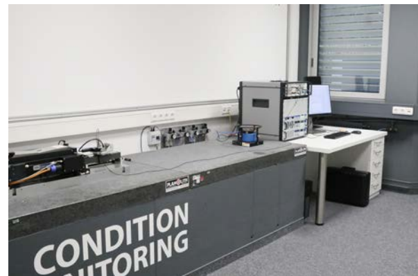
Both shakers are installed on more than seven tons of concrete and granite to calibrate Condition Monitoring vibration sensors with a weight of approx. 50 grams. In the background: high computation power for fastest possible analysis.
