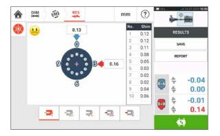
Because vertical motor pumps don't have feet, the angular and parallel adjustment of the motor shaft is made at the motor flange. The angular correction is performed by shimming each bolt position, and the parallel misalignment achieved with jacking screws. Depending on the measurement results, the laser alignment system accurately calculates the required shim thickness and jacking screw adjustments.
