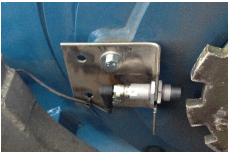
RPM sensor mounted, toothed washer as encoder.
