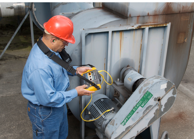
Figure 5. Technician using a handheld vibration analyzer.
