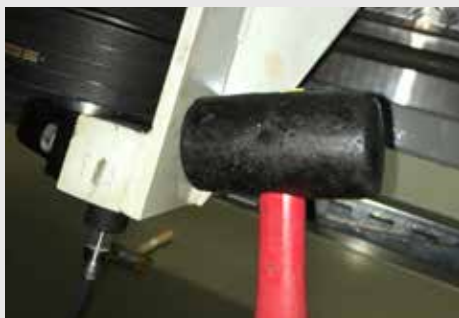
Fig. 2: Bump test on a housing
