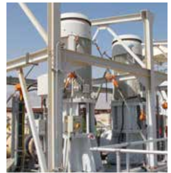
Fig. 1: Simulation of more stiffness with chain-hoists
