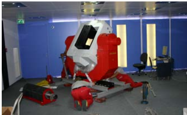
Installing the three-dimensional measurement table in the test laboratory
