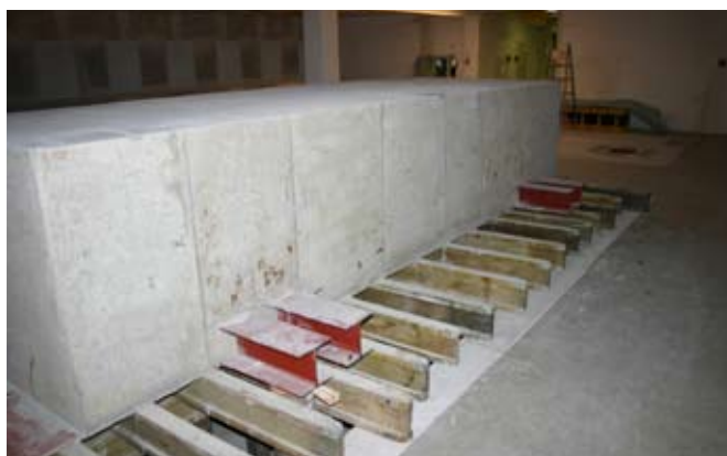
A special concrete mix with steel fibres that cures slowly to counter the formation of cracks
