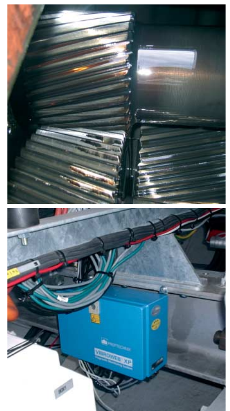
Figure 2: View of tooth damage in a wind turbine gear and a CMS mounted on the main carrier of a wind turbine.
