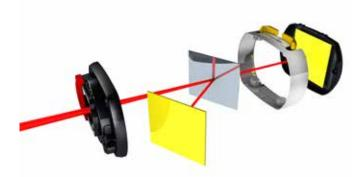
The differentiator behind single-laser technology is located in the sensor housing: A single laser beam is split into two, hitting two separate detectors with an unvariable distance.
