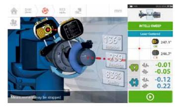
The intuitive user interface supports the user from the beginning to the results stage. In real time, the user can survey the intelliSWEEP<sup>®</sup> process, the measurement quality, and also the physical positions in horizontal and vertical directions of the machine during the entire alignment process.
