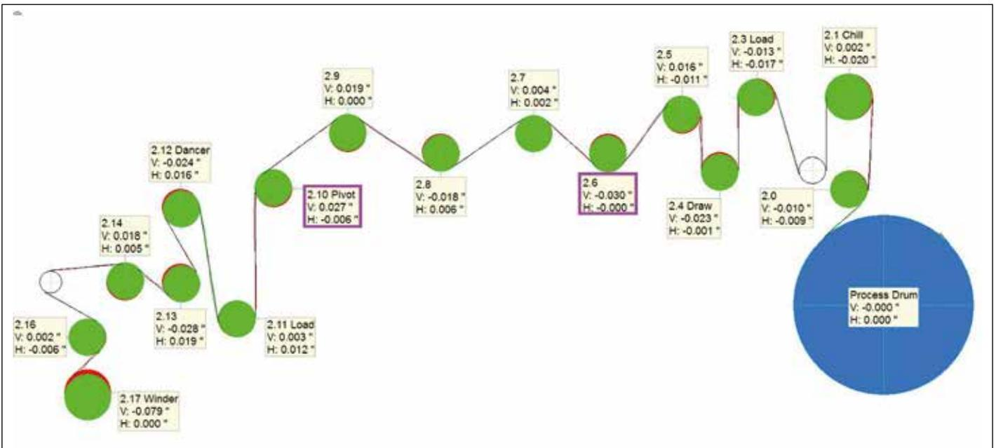
Figure 2.4: Graphical image displaying the final position of the rolls to the left of the Process Drum (reference)
