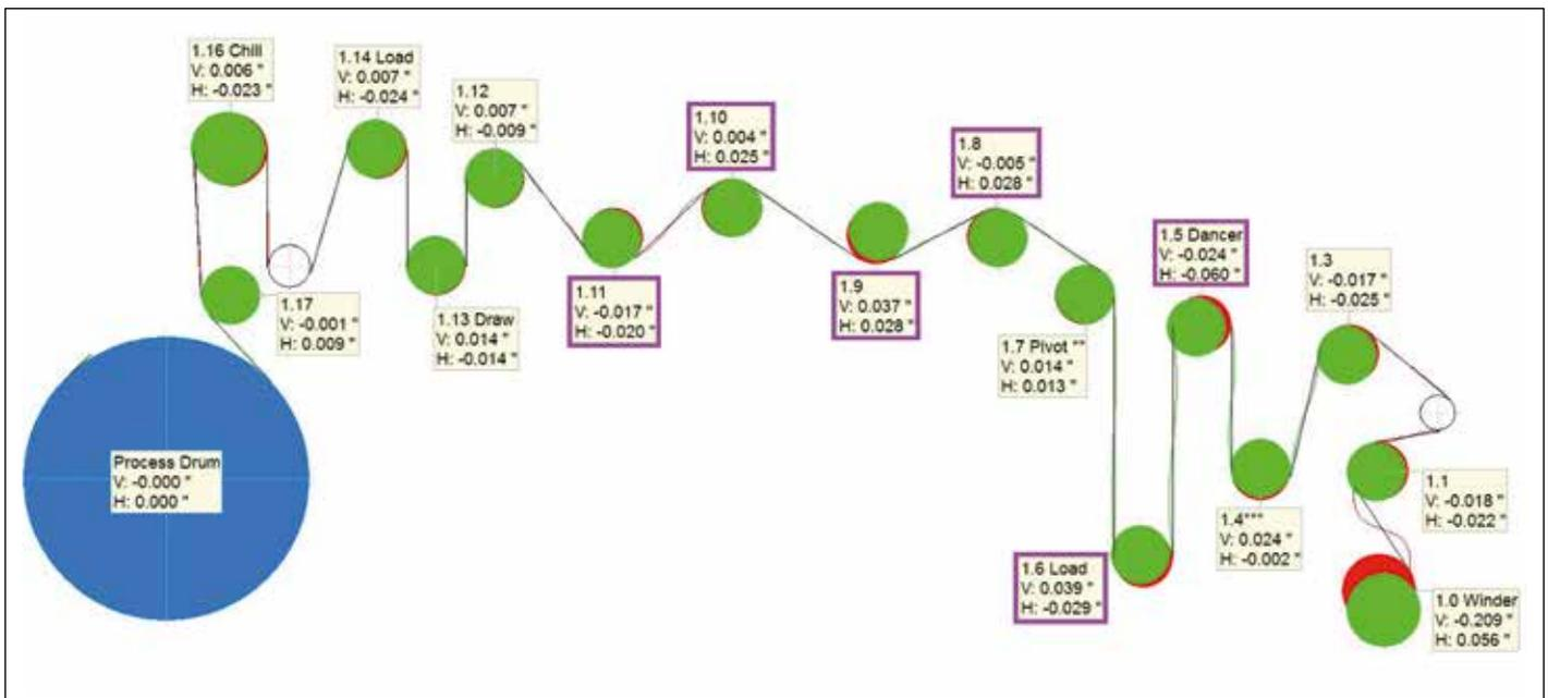
Figure 2.2: Graphical image displaying the final position of rolls to the right of the Process Drum (reference)
