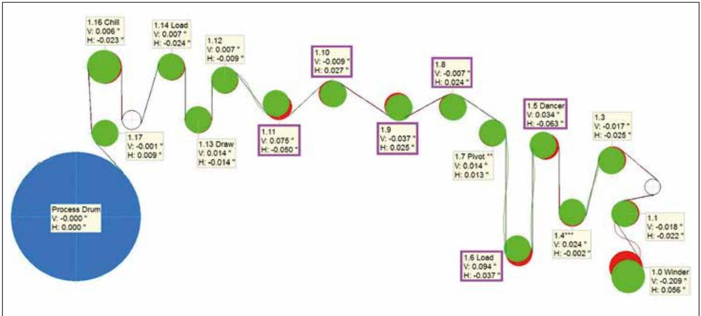
Figure 2.1: Graphical image displaying initial position of rolls to the right of the Process Drum (reference)
