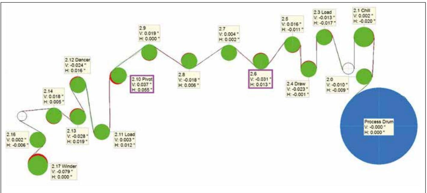
Figure 2.3: Graphical image displaying initial position of the rolls to the left of the Process Drum (reference)
