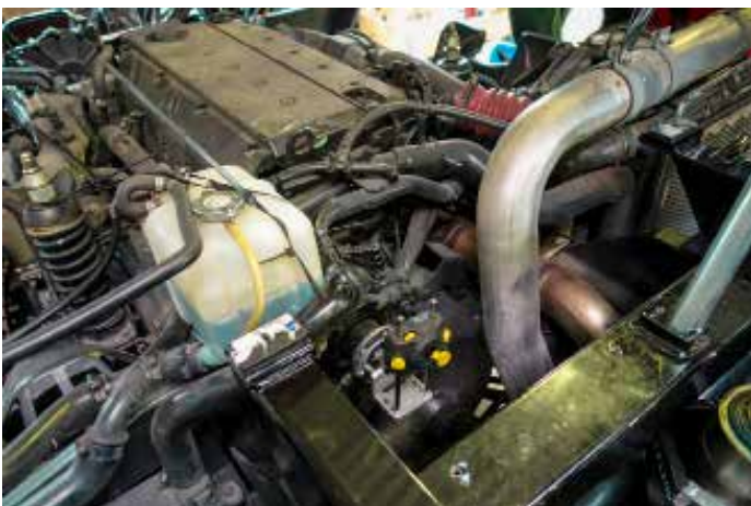
Laser set-up on the gearbox output shaft. The laser has already been set up to record the measurement values.
