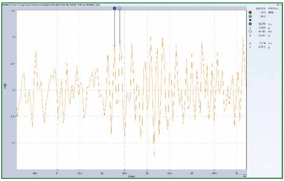
Figure 4b: Zoomed view of the Time waveform accentuating the gear mesh frequency (9.16kHz = 0.11ms) of the bull gear
