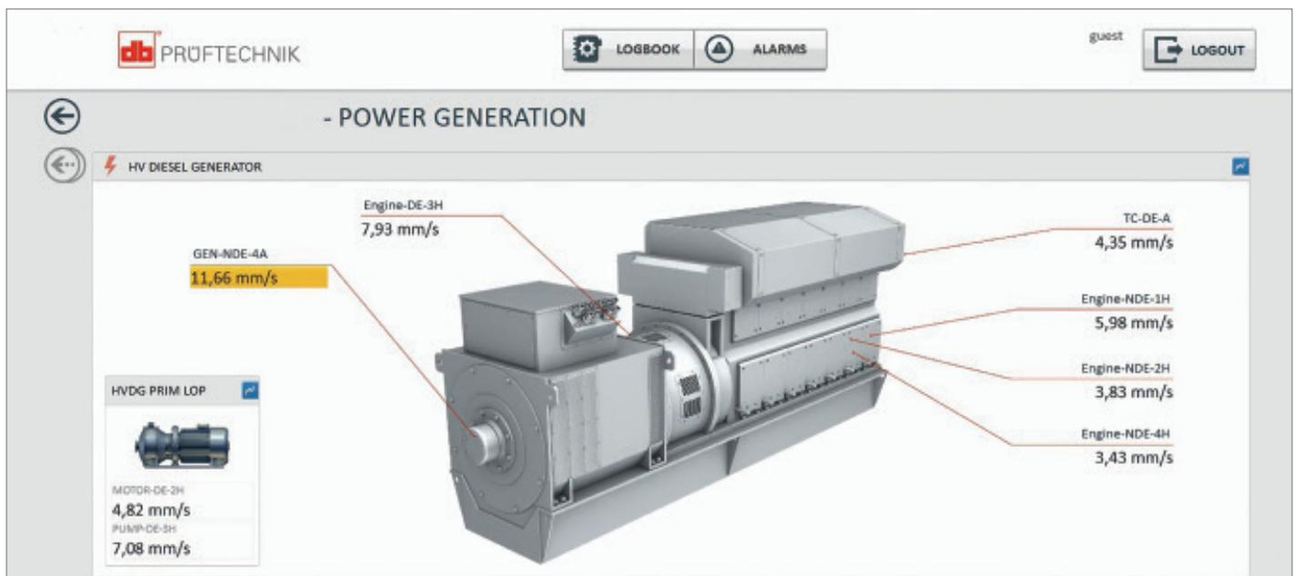
Fig. 2: Drill down to a specific machine train with live data
