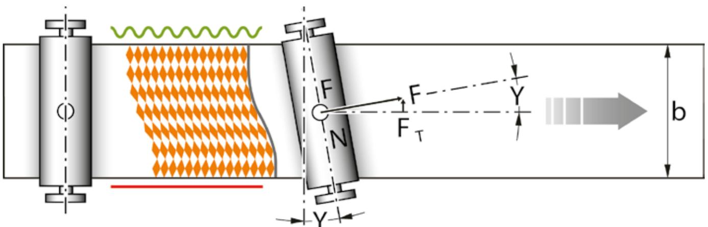
Figure 1: Force distribution due to non-parallel roll alignment
