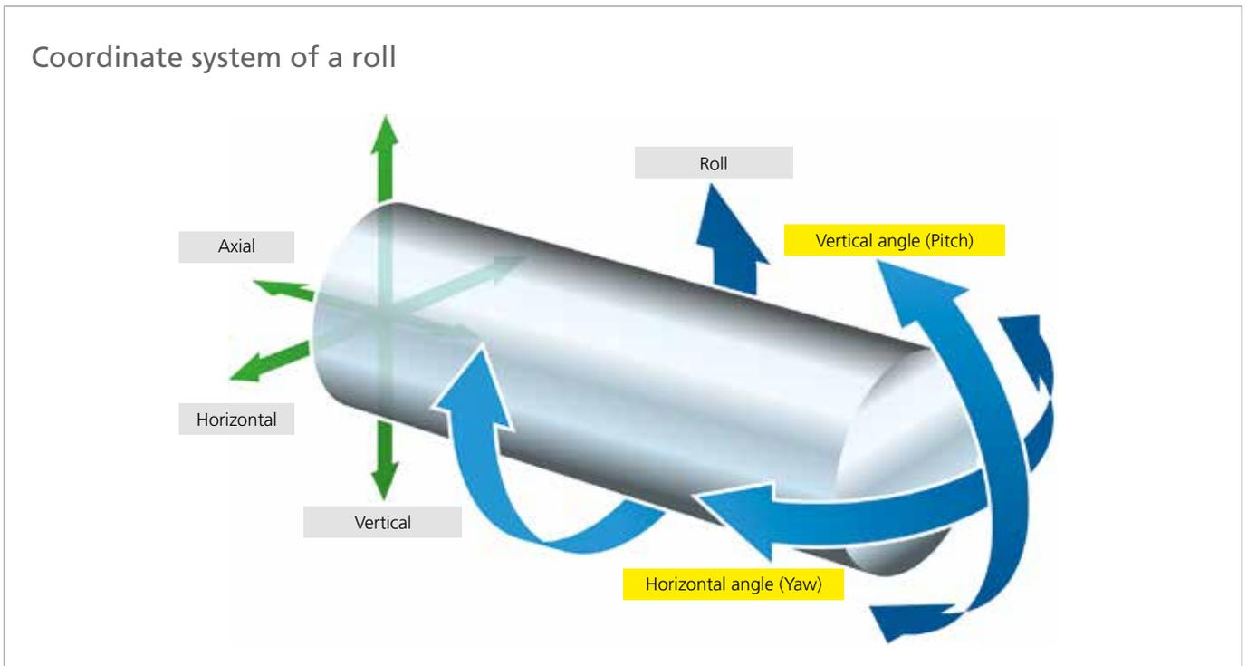
Figure 2: Coordinate system of a roll
