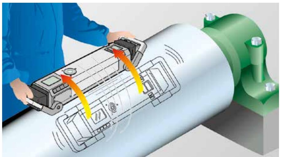
Figure 3: The patented sweep mode: PARALIGN® is moved along a pitch circle on the surface of the roll shell for measured value acquisition.
