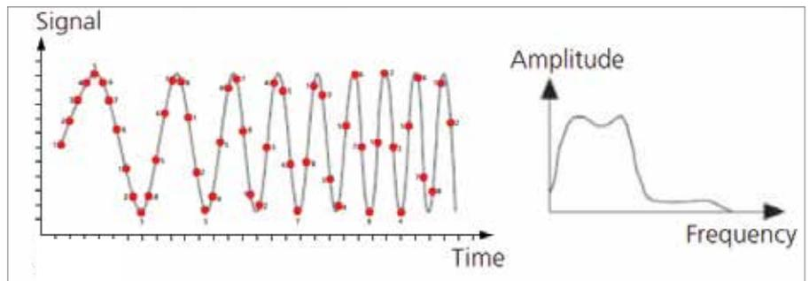
Figure 7: Fixed FFT sample rate resulting in smearing with changing RPM
