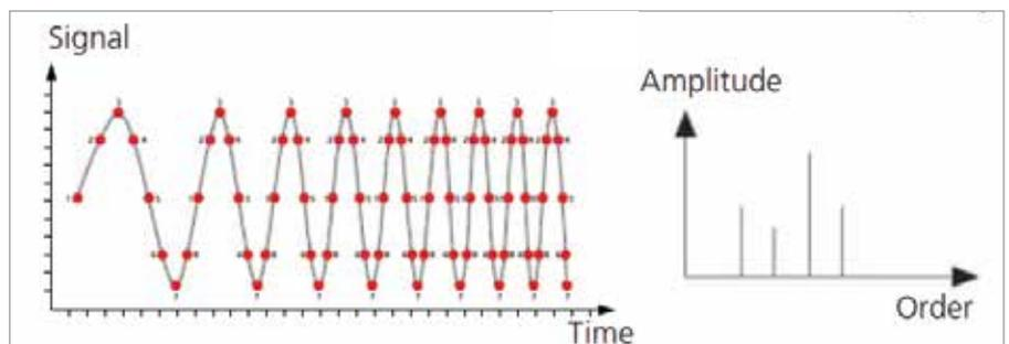
Figure 8: Synchronized sample rate with RPM results in discrete orders
