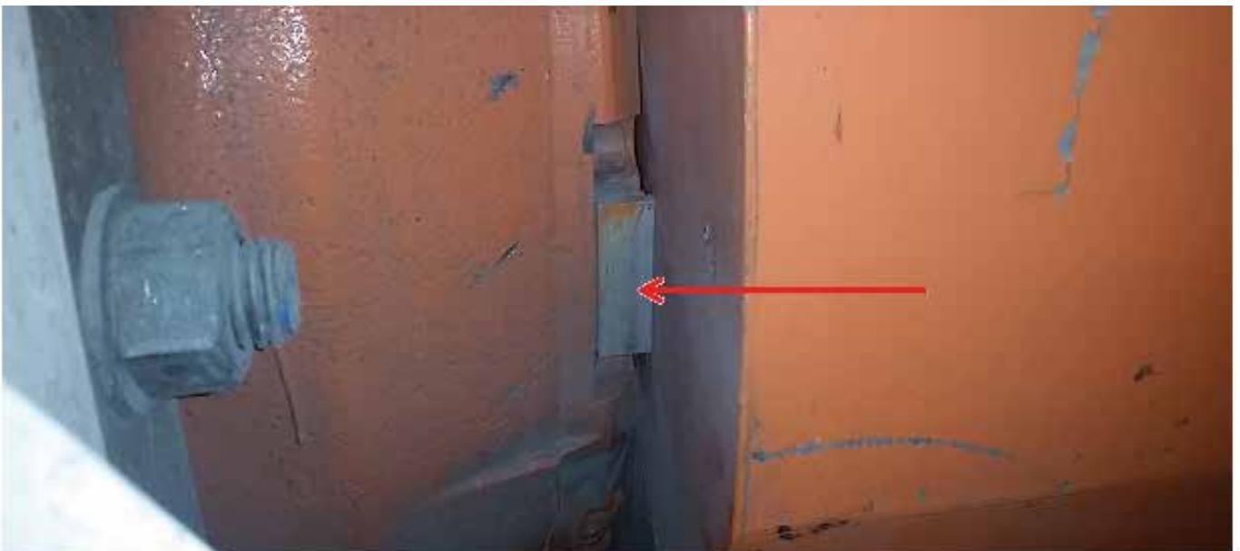
Figure 11: Accelerometer mounting block - DE Motor
