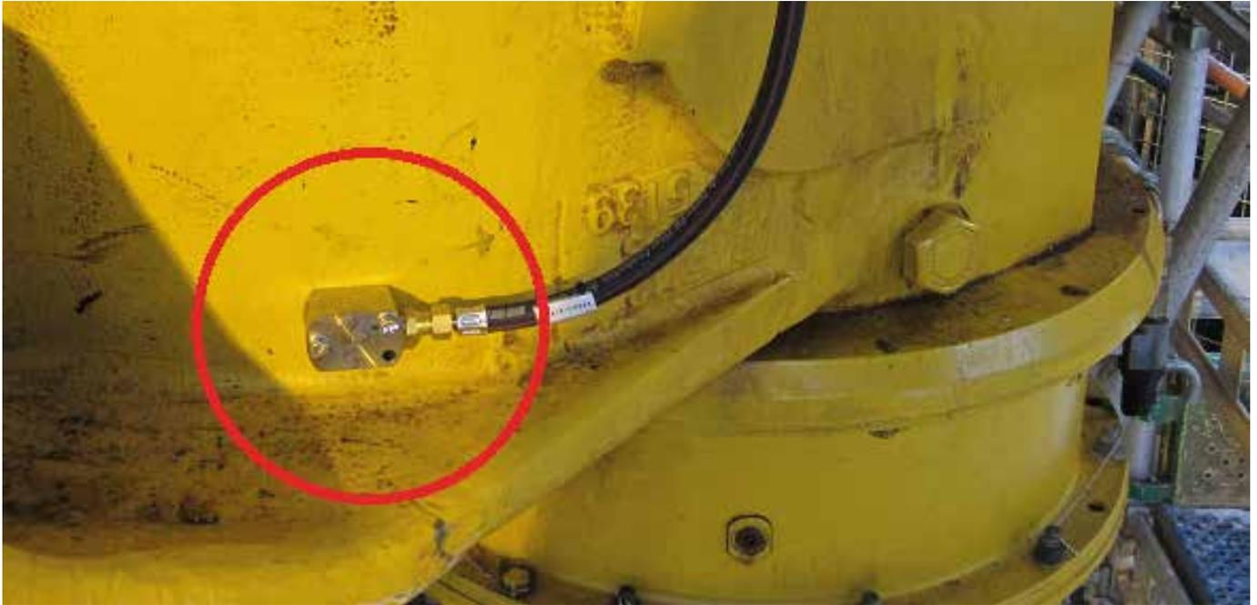
Figure 10: Mini-accelerometer, enclosure and hydraulic hose cable protection
