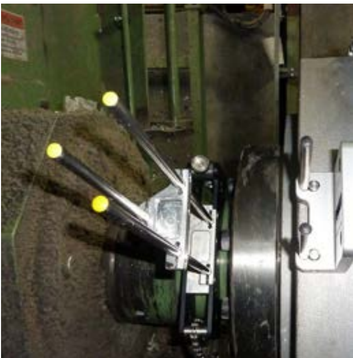
The hexagonal clamp ALI BV 26.x is simply attached to one of the many housing bolts and fastened using a locking pin. The support posts (left) are mounted as usual on the chain-type bracket which is fastened to the shaft.
