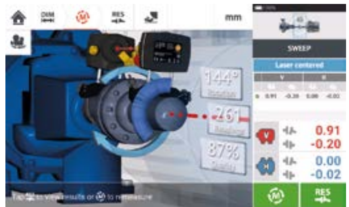
PRUFTECHNIK alignment systems offer the “Continuous Sweep” mode to align precisely shafts.
