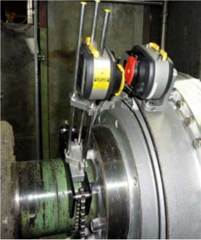
The complete measuring setup including laser and sensor unit protrudes only a few centimeters beyond the fluid coupling. Thanks to PRUFTECHNIK's single-laser technology, the distance between laser and sensor does not influence the measurement result.
