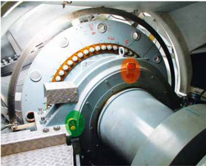
Image 3 (left) and 3a (right): Views of the mounted laser sensors, in order to record displacements, movements and tilting of the drive train components in relation to each other
