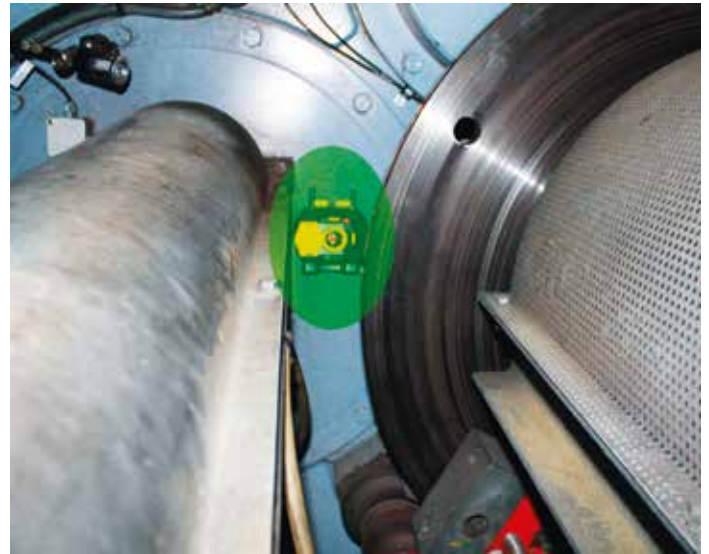
Image 3 (left) and 3a (right): Views of the mounted laser sensors, in order to record displacements, movements and tilting of the drive train components in relation to each other
