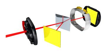
The differentiator behind single-laser technology is located in the sensor housing: A single laser beam is split into two, hitting two separate detectors with an unvariable distance.
