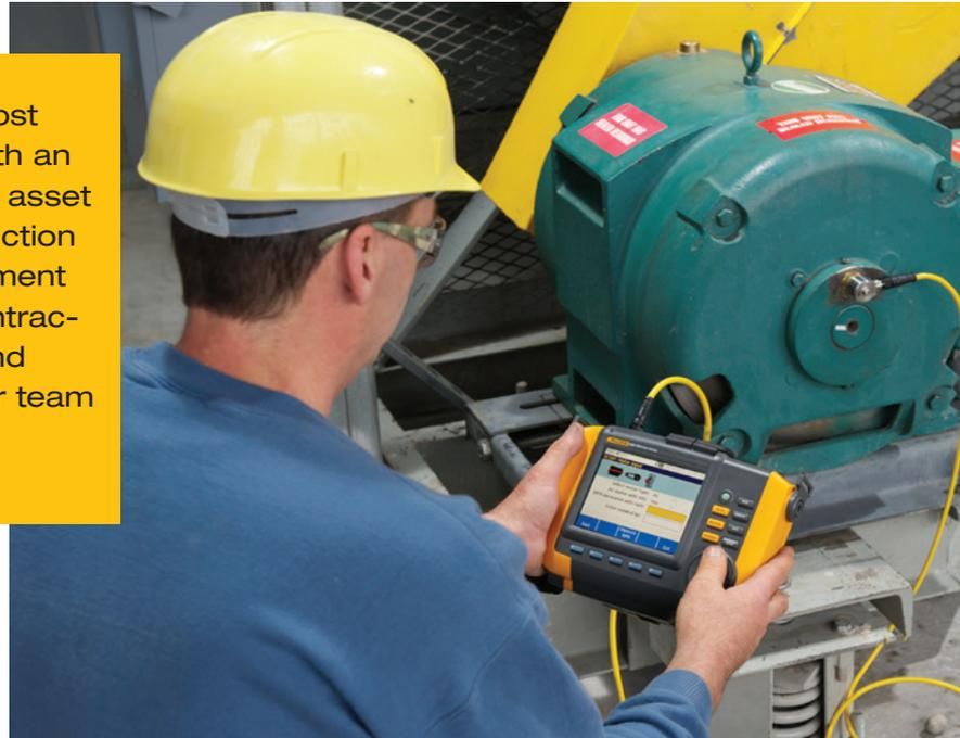
The 810 Vibration Tester monitors an operational motor.
