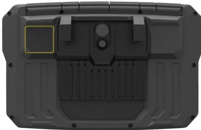
Identification is done with provided RFID tags. The tag is attached to an asset. To read the tag place the device reader module as close as possible to the tag (to within 5 mm if possible)
