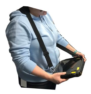
Use the buckles to adjust the length of the hand straps. When the size of the hand straps is correct, use the Velcro fasteners to wrap the straps. This gives you a reliable and comfortable grip.
