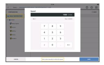
This option is used when an RPM sensor is not available and there is need to measure an asset that requires the RPM. Examples include roller bearing condition and order-based spectra.
