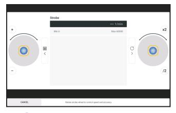
Tap or press device ENTER button (either of the two yellow buttons on the device) to turn the stroboscope on.
