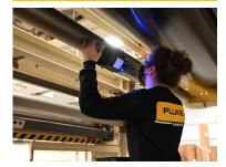
Suitable for measuring roll misalignment that can cause inefficiency and quality issues
