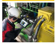
Suitable for measuring rotating axes of coupled shafts in various sizes and length
