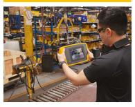
Suitable for detecting leaks in air or gas pipes and vacuum systems
