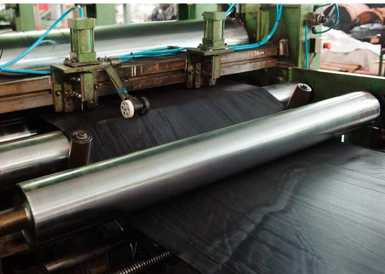
Misalignment of rolls on a tire line eventually leads to costly problems such as poor tracking, stretching, wrinkling, uneven coating, and ultimately, product defects.
