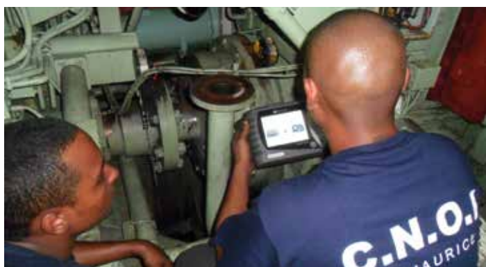
Shaft alignment measurement using the ROTALIGN® Ultra iS platform
