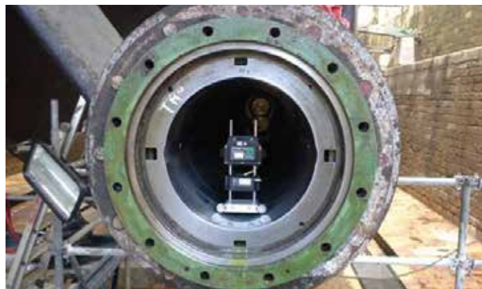
ROTALIGN® sensor positioned in the stern tube
