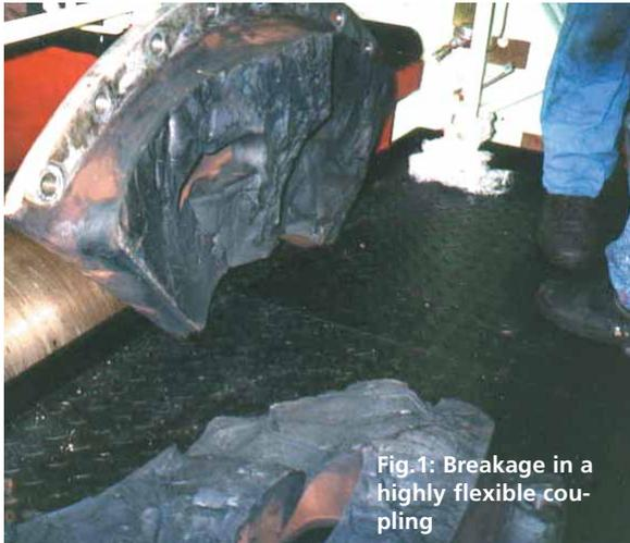
Fig.1: Breakage in a highly flexible coupling
