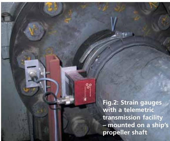
Fig.2: Strain gauges with a telemetric transmission facility – mounted on a ship's propeller shaft
