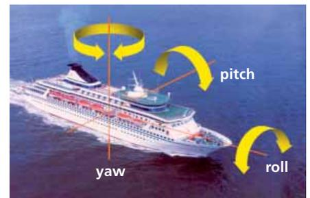
Fig.1: Typical ship vibrations
