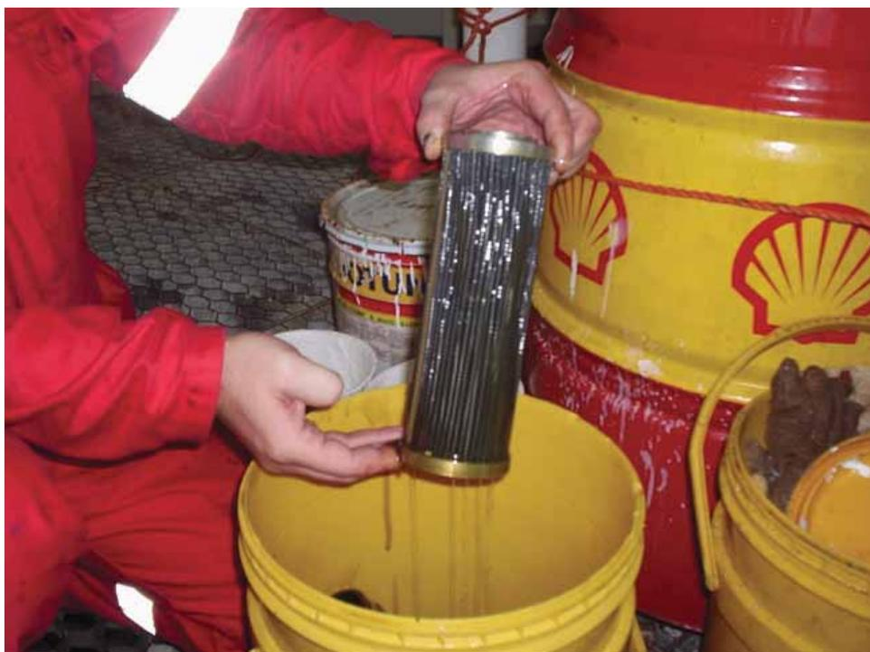
Fig. 1: Condition analysis of oil filter after removal
