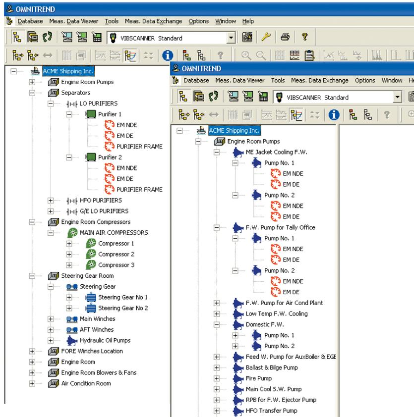
Fig.3: The tree structure in the OMNITREND® software shows all components monitored on the ship
