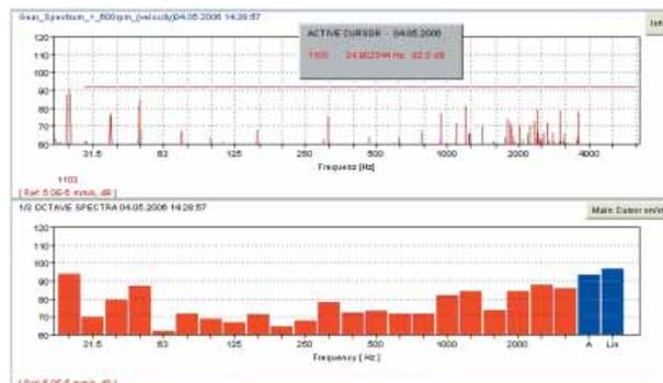
Fig.3: Third octave and narrow band spectra of an acceptance measurement
