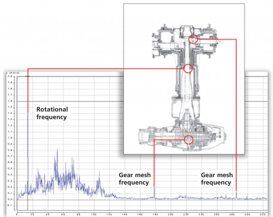
Fig.4: The velocity spectrum showed increased excitation of the long spacer shaft
