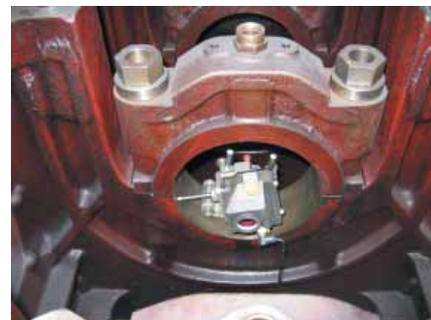
Fig.2: The laser sensor, which can be rotated inside the bore
