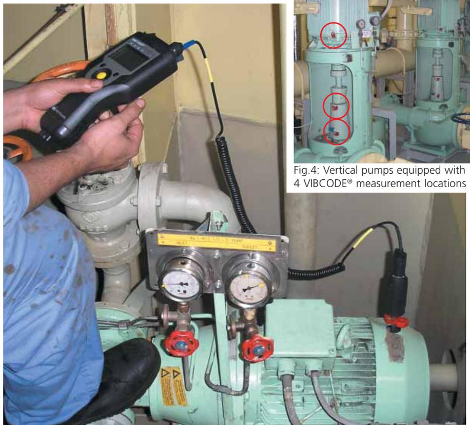
Fig.5: Offline measurement on the ventilator side of the motor bearing using VIBSCANNRT®
