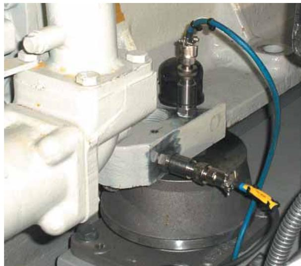
Fig.2: Accelerometers installed on a diesel engine base
