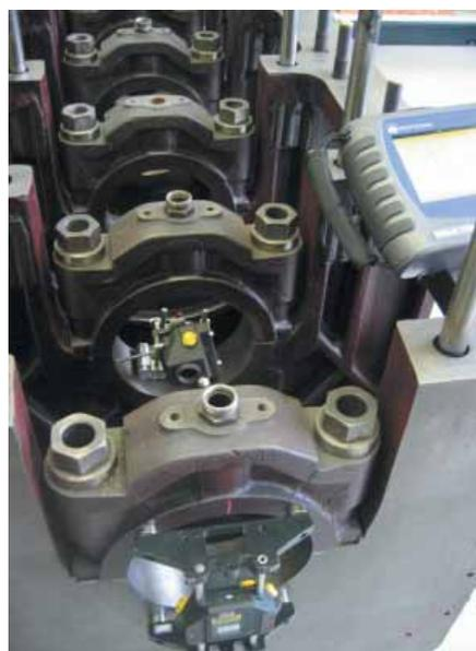
Fig.1: Laser equipment for monitoring the bearing saddles
