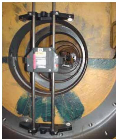
Fig.3: The laser transmitter with magnetic mounts
