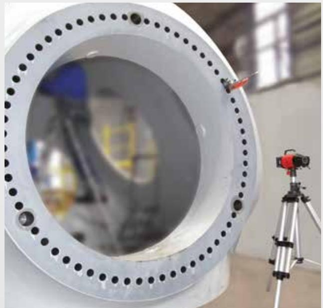
Measurement of flange flatness using LEVALIGN® expert.
